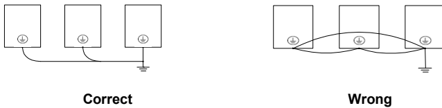
Fig. 3–3 Grounding wiring
