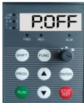
Fig 3-1 Power-on Parameter Display Initialization Display "P.OFF"
