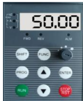
Fig 3-2 Stop Status Parameter Display Set Frequency "50.00"
